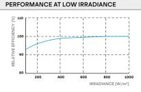
Typical module performance under low irradiance conditions in comparison to STC conditions (25  $^\circ C,\,1000\,W/m^2)$
