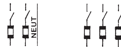
Three-wire SN, 240 volts ac
