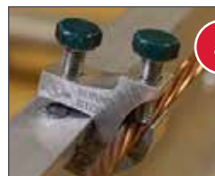
3 THIN WALL C-TAPS Type YC-L is a thin wall, high conductivity copper connector for making copper taps and parallel connections for #14 for 3/0 AWG
